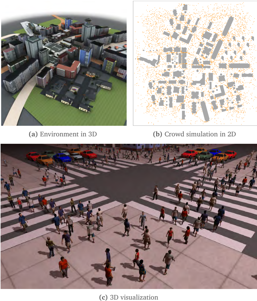
Figure 1.1: Example of a crowd simulation in a virtual environment. (a) The original 3D model of the environment. (b) For crowd simulation purposes, this environment can be simplified to a 2D representation with polygonal obstacles. Characters in the simulation are shown as orange disks; we have enlarged these disks for clarity. This figure was generated using our crowd simulation framework from Chapter 10. (c) The simulated characters can be visualized as animated 3D models in the original environment [65].
